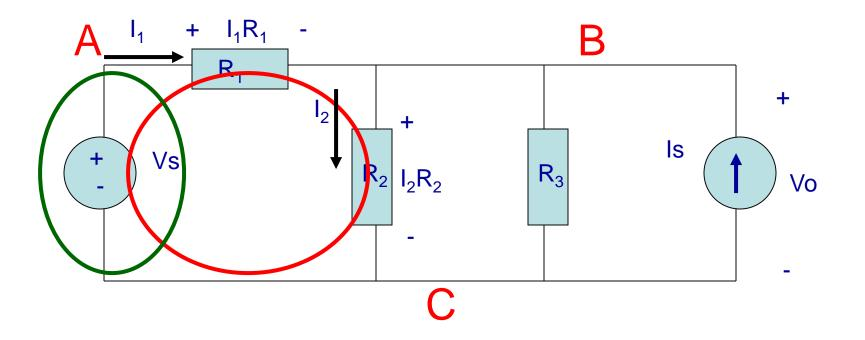
Subtract the voltage rise from C to A through Vs:  $+I_1R_1 + I_2R_2 - Vs = 0$ Notice that the sign of each term matches the polarity encountered 1st
