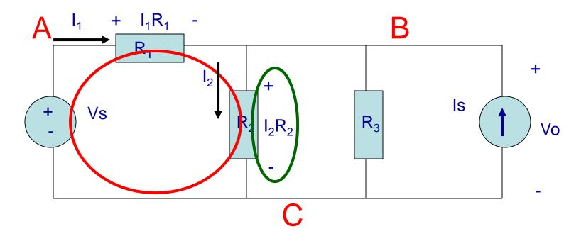
Add the voltage drop from B to C through  $R_2$ : +  $I_1R_1$  +  $I_2R_2$
